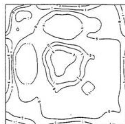
Fig. 13. Two residuals shows the roughness effect. (a) and (b) are the results of roughness parameters of 1000 and 10, respectively. Tension parameter is fixed at 0.
